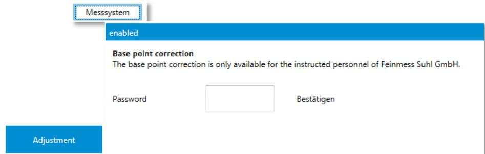
This menu can only be achieved in the “measuring system” channel, since this impacts the accuracy of the measuring system.
