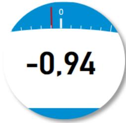
The digital measured value displays the offset or the individual channel measuring value.
