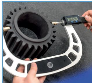
0806 Digital micrometer with pins to fix balls or rollers
