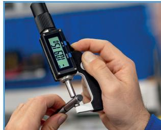
0800Lift Digital micrometer with lifting knob for serial measuring
